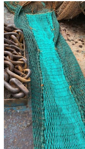
Figure 4 Image of a sheet of luminous netting fitted on the bottom panel of the SELTRA270 section. The trawl has been turned inside out in the photograph to allow fitting of the new netting.
